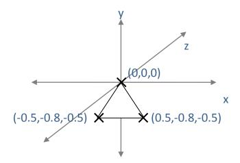
As well as the X, Y, and Z-axis position, vertices can each have a color which contributes to the color of the associated primitive. If you do not set a color on the vertex explicitly, the color black is used.
